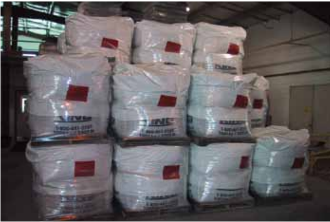
A clean, level, designated storage area should be chosen for shotcrete, preferably with protection from the elements.
