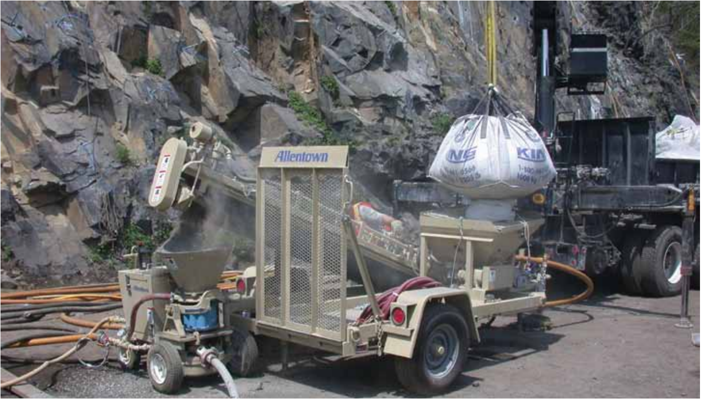
Pre-dampening will greatly reduce the amount of airborne dust at the machine and at the nozzle, and will eliminate static electricity build-up in the hose.
