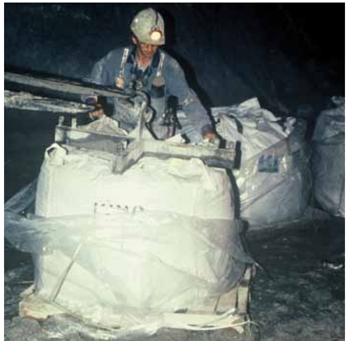
Always suspend a bulk bag from all four corner-lifting straps.
