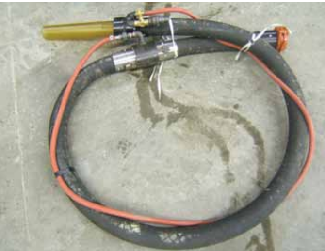
If a pre-dampener is not used, ensure that a hydro-nozzle or semi-wet nozzle (one in which the water ring is moved back several feet in the hose) is used.
